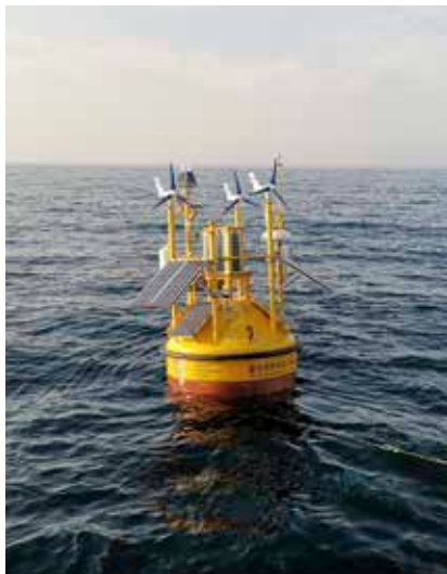
Floating LiDAR system
