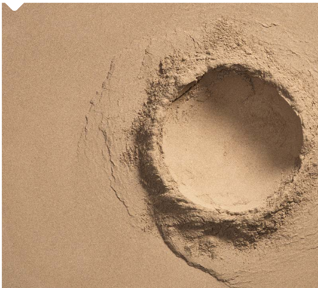
Secondary material, M&W, FORZ® Filler, made from tar and polluted soil
